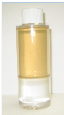
CAO-46 GR lubricants resist water contamination, typically separating in two distinct layers.
