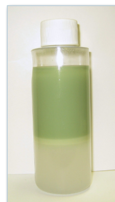
OEM PAGs like Sullube often form an emulsion when contaminated by water.
